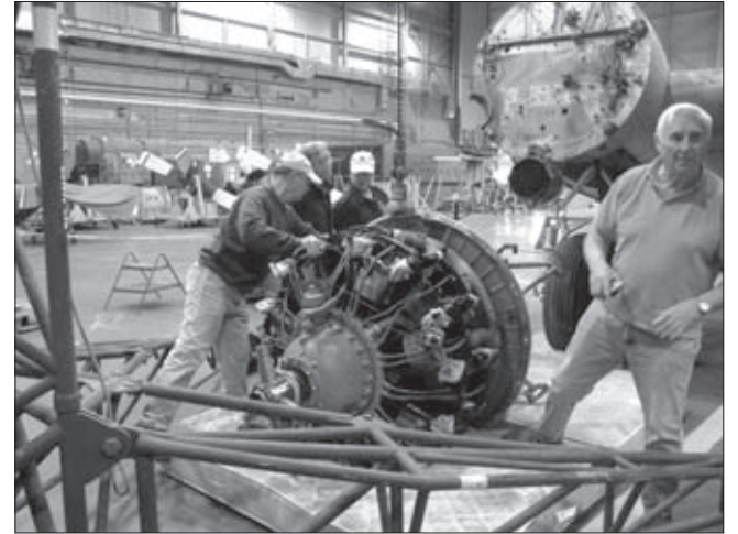
Doc McKeil, Eric Welin, Brian Troniak and Bill Flinn prepare the starboard engine for mounting on the wing box. (Images: Dave Richards)
