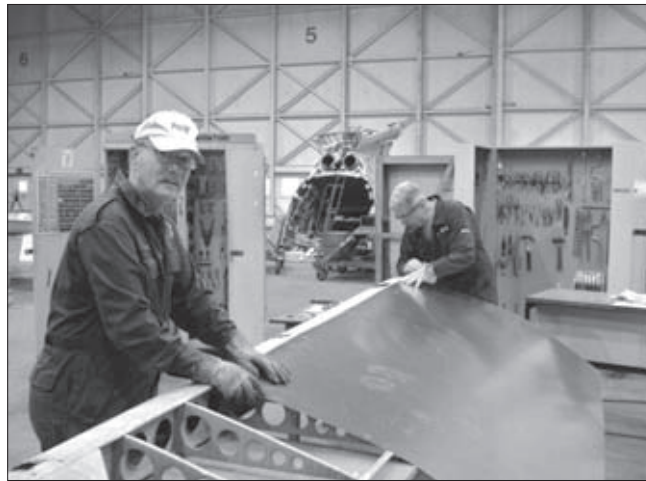
Doc McKeil and team leader Eric Welin installing aluminium panels on flaps replacing fabric.
