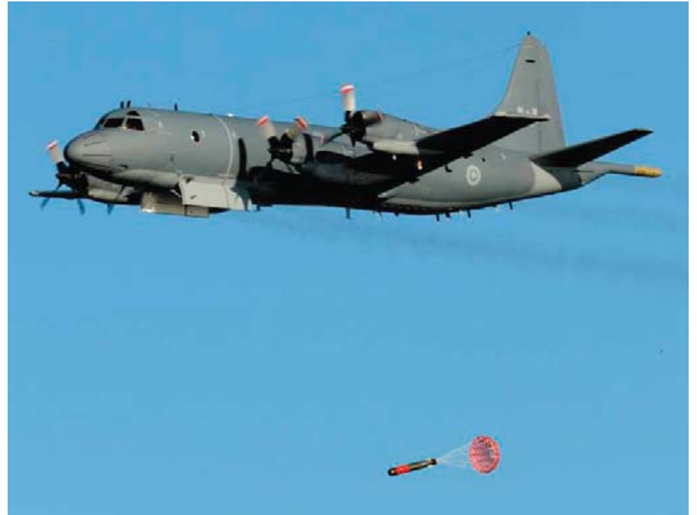
Testing in Comox checked the Block 3 weapon system's performance when dropping torpedoes.
