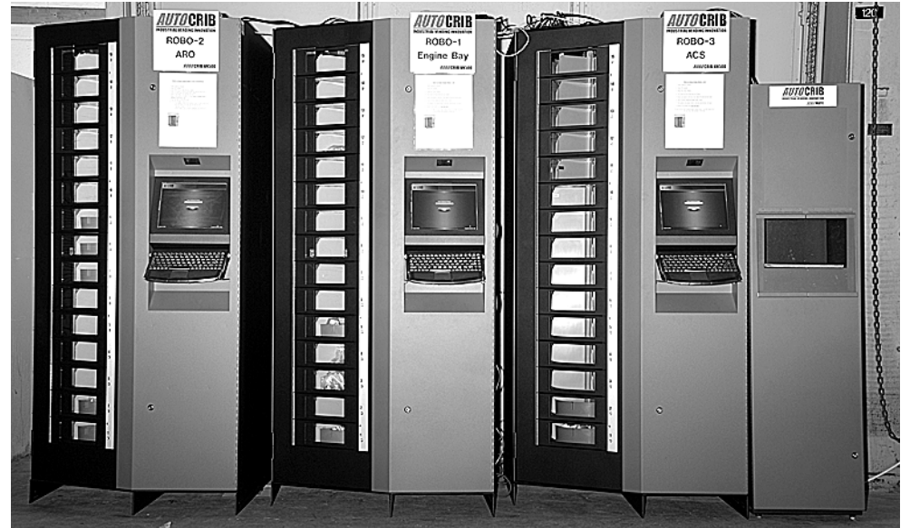
Three new "vending machines" are supplying 14 Air Maintenance Squadron maintainers with at-hand parts, right on the hangar floor. Submitted
