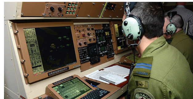
The new Block III operational mission simulator flight deck training station and instructor operation stations, manned by operators and system engineers.
