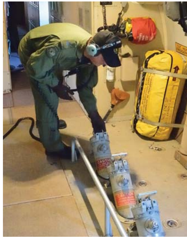
Master Corporal Ulrich (Pim) Reiner, an airborne electronic sensor operator with 405 (Long Range Patrol) Squadron, conducts preflight checks on a sonobouy launch tube September 16.
