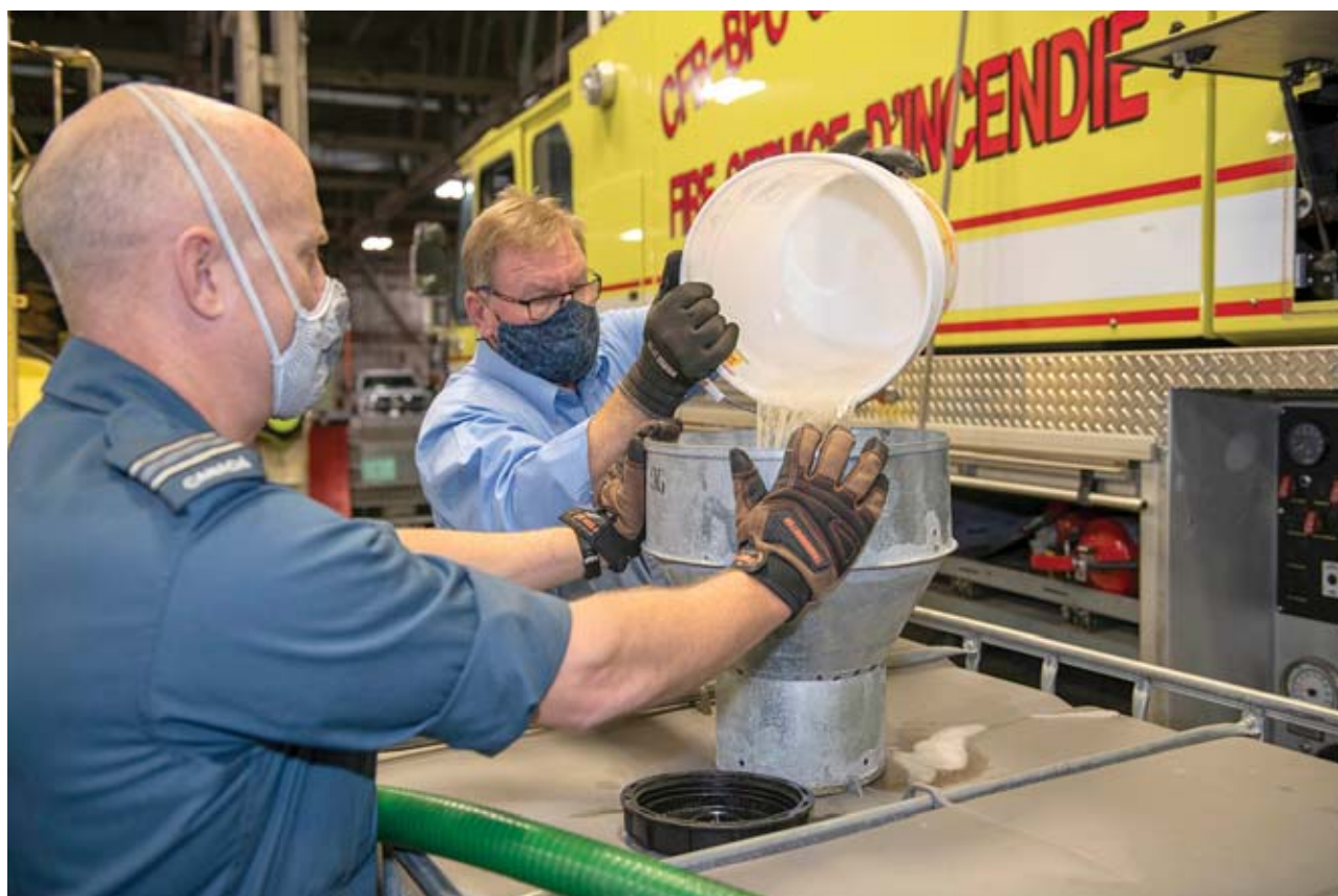
14 Wing Greenwood, Department of National Defence environment and contractor personnel ran a week-long trial in November, flushing a military fire truck and testing for residual polyfluoroalkyl (PFAS) contaminants.
