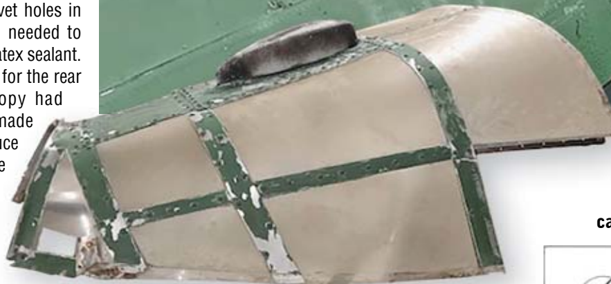
The make-shift aft canopy, removed from the Greenwood Military Aviation Museum's display Avro Lancaster for winter work.
